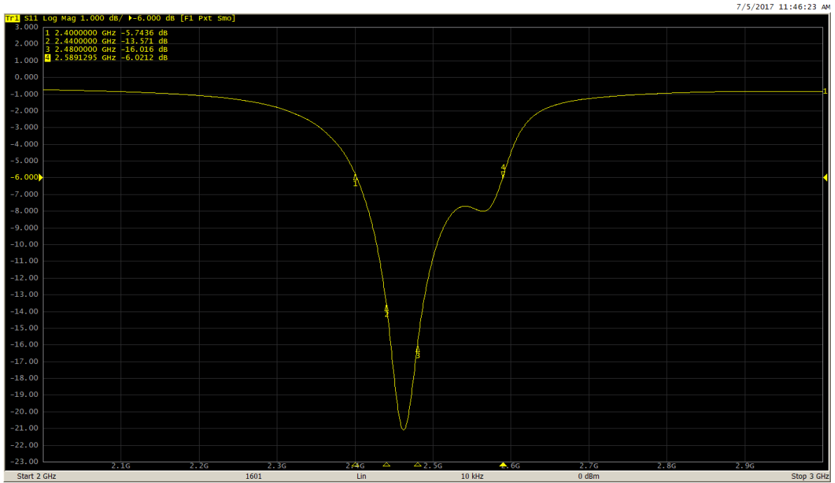
Figure 3: Return loss measured on a 0.35 mm thick, 100 x 100 mm brass plate
