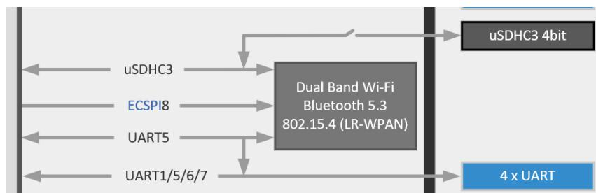
**Figure 3: VAR-SOM-MX93 Wi-Fi Module Internal Connection**
