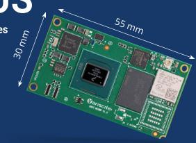
The DART-MX8M-PLUS provides various interfaces and connectivity options: certified dual-band Wi-Fi 802.11ac/a/b/g/n, BT/BLE, dual GbE, dual USB3, PCIe, SPI, and UART.
