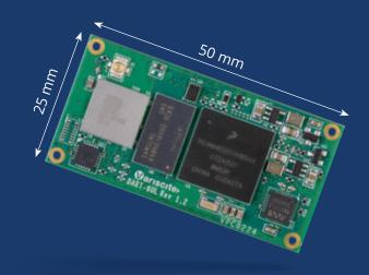
The DART-6UL highly integrated connectivity includes a certified WiFi, Bluetooth/BLE, dual Ethernet, dual USB, audio, display with touch panel and serial interfaces. In addition, the system supports industrial operating grade, targeting embedded application requiring a wide temperature range.
